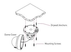
4. Fix the dome cover back onto the mounting base by installing the three dome cover screws into the camera and tightening it once the position is secured.
